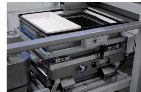
Picture 7: Weigher in a weigher. The combination of two weighing hoppers of different sizes allows for accurate dosing over a wide range of weights. Source: ALFRA
